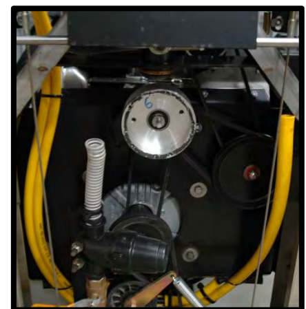
FIGURE 3: Pump removed from the T3000i. Black RTV silicon is also visible on the hub ring.
