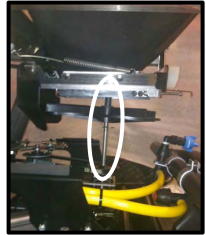
FIGURE 1: Spinner Shaft not perpendicular to level
