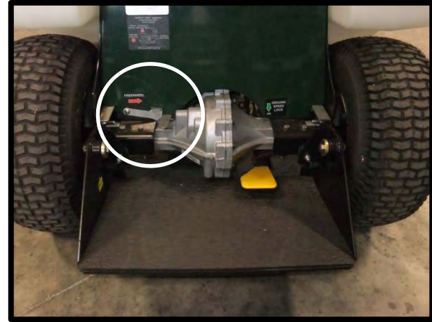
FIGURE 4: Place the T3000i in freewheel to open the transaxle bypass valve.
