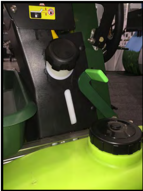
FIGURE 7: Translucent fuel tank
