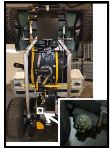
FIGURE 2: Crown nut location
