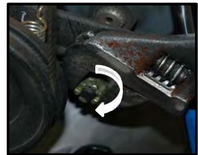
FIGURE 3: Tightening the parking brake
