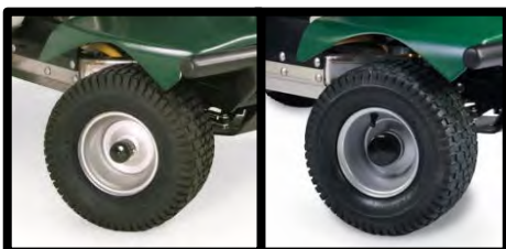
FIGURE 3: Left) Old front wheel bearing, Right) New front wheel bearing
