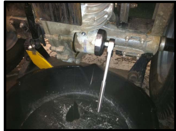
FIGURE 1: Transaxle oil filter being removed from the transaxle
