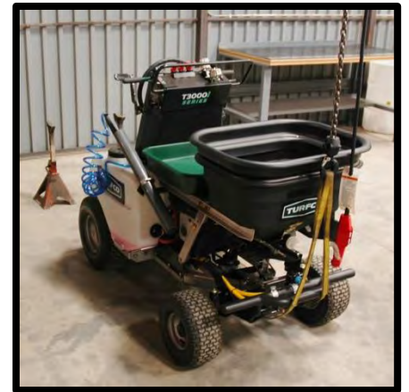
FIGURE 2: Lifting device attached to T3000i
