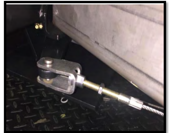
FIGURE 5: 2015 & Newer units adjustable clevis
