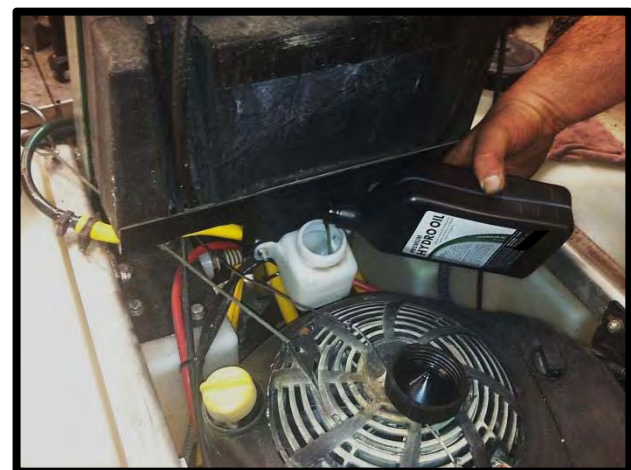
FIGURE 3: Filling the remaining oil in the transaxle oil expansion tank
