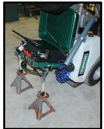
FIGURE 3: Jack Stands Supporting T3000i
