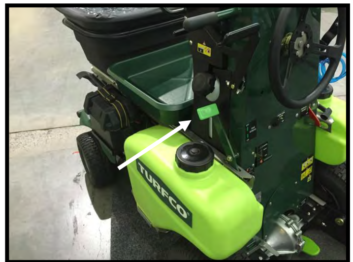
FIGURE 8: New solid linkage trim lever
