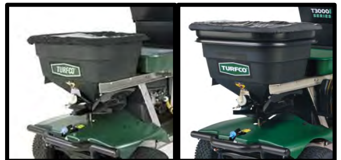
FIGURE 4: Left) Old 120lb hopper, Right) New extended 175 lb hopper
