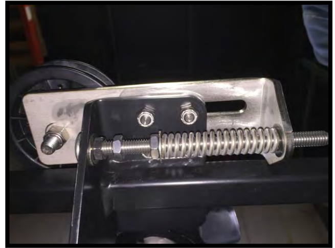
FIGURE 5: New idler pulley system
