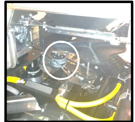
FIGURE 2: Variable Speed Pulley
