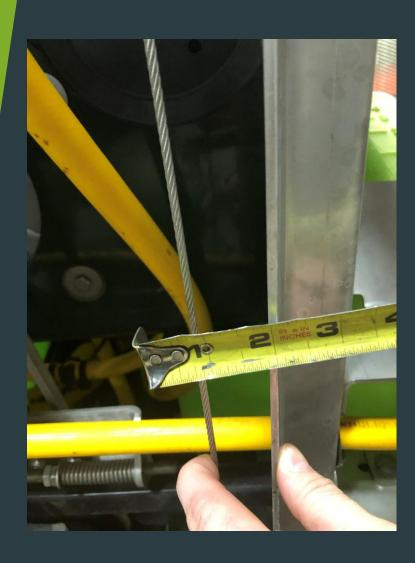
Step 2: Push steering cable towards frame to take measurement
