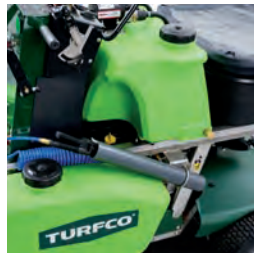
Optional T-Flex15 tank offers the ability to cover up to 140,000 sq. ft. per fill and spray two liquids simultaneously or independently.
