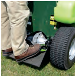
Hands-free speed control allows operators to manage other functions without stopping, such as utilizing the spot treatment wand or other spray/ spread controls.
