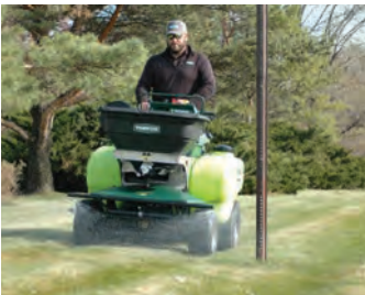
Unique two-nozzle boomless spray system delivers an industry-leading spray width of up to 10 feet.
