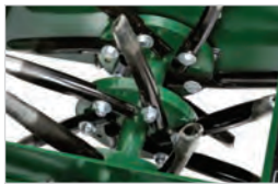
Patented EasyChange tines can be quickly accessed and replaced.
