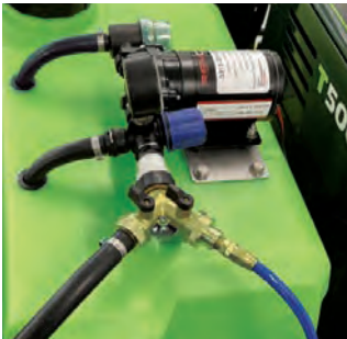
Brass, threaded, control valves to adjust flow rates or switch between wand and front spray nozzle.
