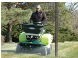
Unique two-nozzle boomless spray system delivers an industry-leading spray width of up to 13 feet.
