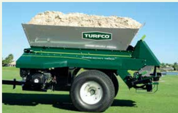
*Widest hopper in the industry fits an 80" bucket — minimizes spillage.*
