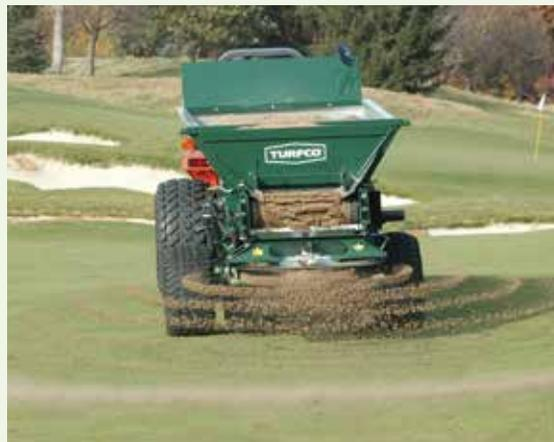
Light, medium and heavy spreads from 15 to 45 ft wide with WideSpin technology.
