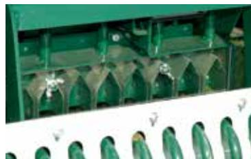
Patented seed diverter increases germination by placing seed directly into the slit.
