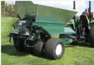
Four-wheel walking beam suspension.
