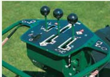
*A control panel for operator convenience features forward and reverse, brakes and fingertip throttle control.*
