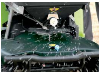
Specially molded, hard trim design reduces cleanup and wasted fertilizer.
